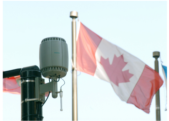
BelAir's high performance wireless mesh technology is used for Toronto's Wi-Fi zone
